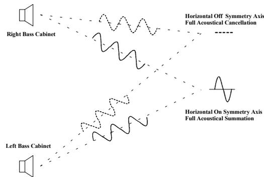
Fig. 6. Two bass cabinets with large horizontal distance. Large travel distance differences lead to almost full cancellation for certain frequencies off symmetry axis
