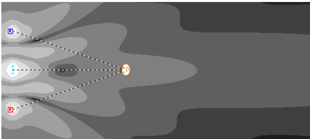
Fig. 19. Horizontal coverage of Left-Center-Right bass arrays
