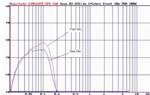
Fig. 1. Frequency response of a typical 18" vented cabinet. Measurement shows front vs rear radiation. Crossover frequency 124Hz, Linkwitz-Riley 24dB/Oct.
