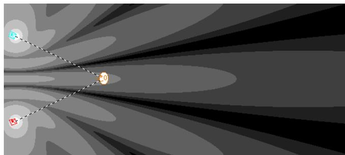
Fig. 7. ‘Bass Alleys’. Two bass cabinets with 10m distance. Horizontal coverage at 100Hz
