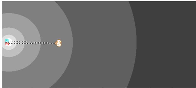
Fig. 9. 1-by-2 Array horizontal coverage at 100Hz. Two 90cm\*60cm Bass cabinets side-by-side
