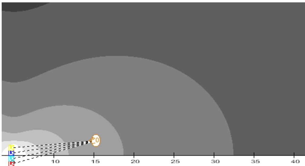
Fig. 14. 2-by-4 Array at 100Hz with mirror cabinets. Vertical coverage. Side view
