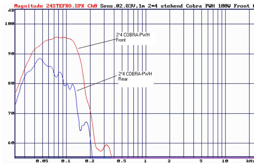
Fig. 17. Front vs back radiation of a 2\*4 tightly packed bass array
