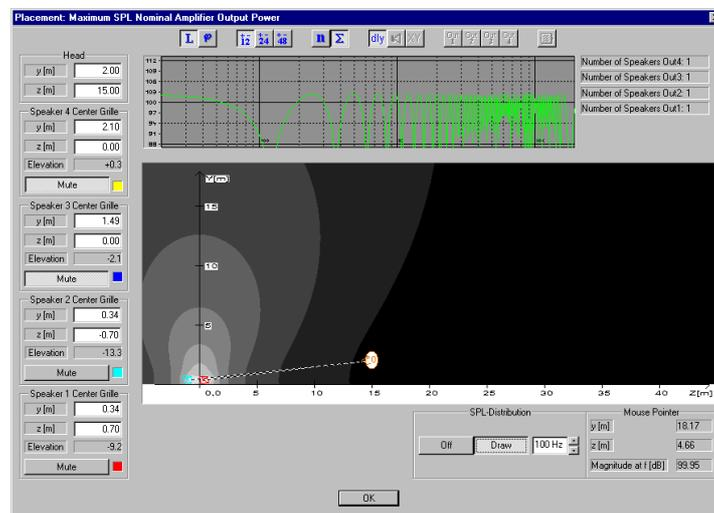
Fig. 5. Idealized cabinet with 70 cm depth placed against a wall at 100Hz (shown with mirror cabinet)
