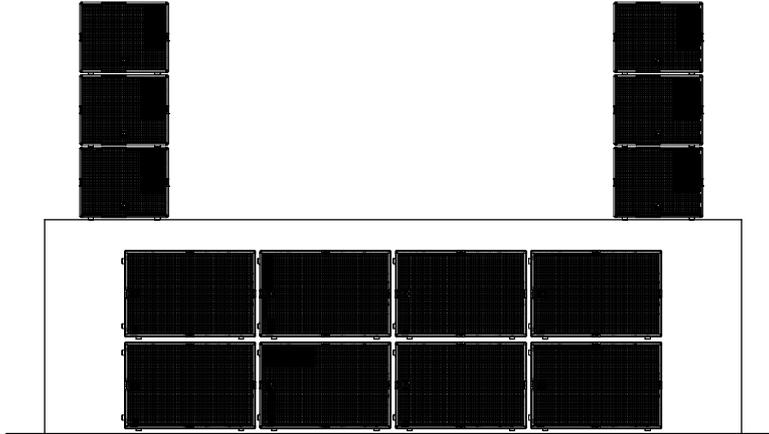
Fig. 15. 2-by-4 Bass array together with mid-high cabinets on the stage
