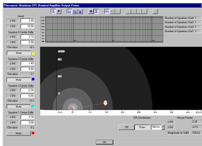
Fig. 3. SPL and directivity of an omnidirectional point source without any reflecting surface, 100Hz
