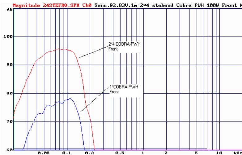
Fig. 16. Comparison of the frequency response of a single 18" vented cabinet vs an array of 2\*4 cabinets.
