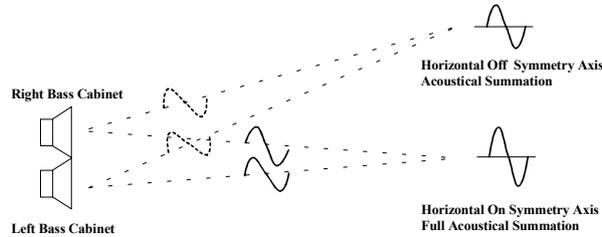
Fig. 8. Two bass cabinets placed side-by-side. Only small travel distance differences for low frequencies
